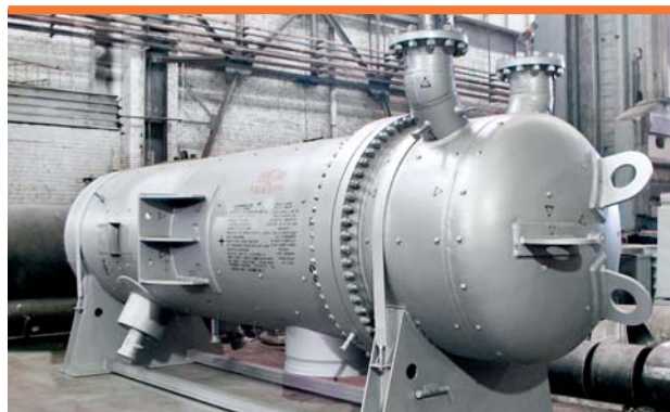
Low pressure heaters manufactured by ZiO-Podolsk are successfully operated at CHPP-27 of Mosenergo as a part of PT-80 (Russian: ПТ-80) turbine group.
