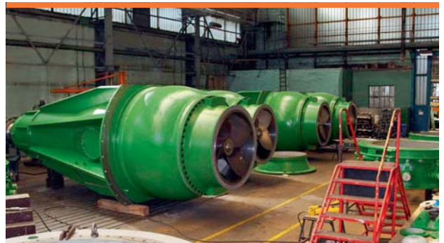
Axial and angular-flow single-stage semi-submersible with regulation system of hydraulic characteristics pumps
