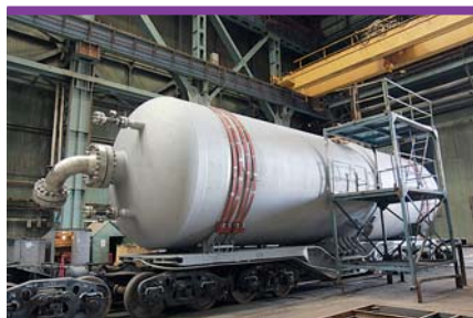
Hydrotreater for Ryazan refinery
