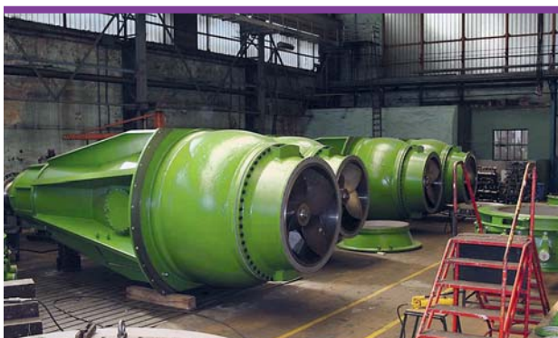
Axial and angular-flow single-stage semisubmersible pumps with regulation system for hydraulic characteristics
