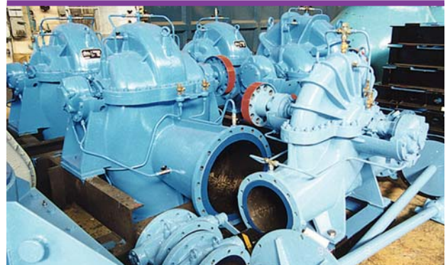
Horizontal centrifugal ones with double inlet impeller with a horizontal and a vertical split
