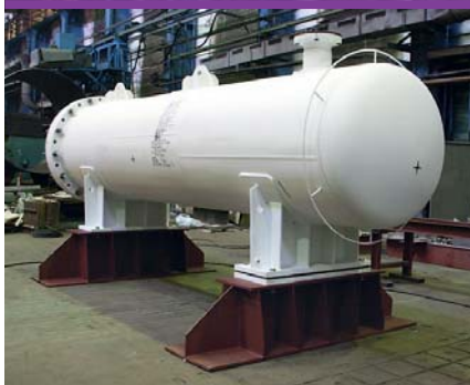
Heat exchanger for Sakhalin II project (fully compliant with ASME code requirements)
