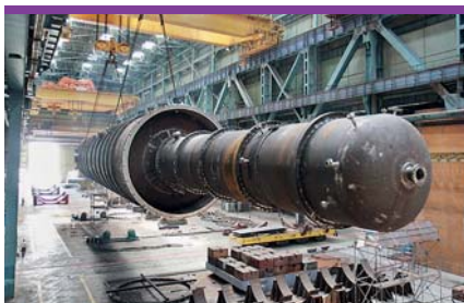
67 m long column, weigh 346 tons for JSC Taneko
